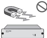
Electronic elements including capacitance and inductance on the device can be affected by external interferences, such as conducted emission by capacitance coupling, inductance coupling, and impedance coupling. To decrease the interferences, please make sure to take the following measures:
