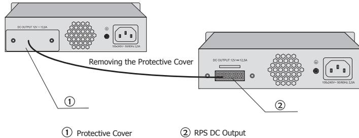
Figure 3-2 Removing the RPS Protective Cover
