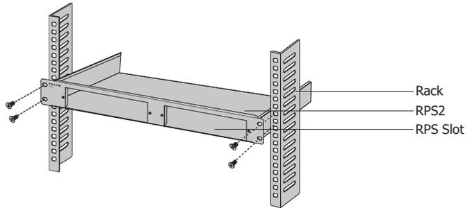
Figure 2-2 Install the RPS2 to a standard rack
