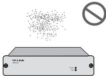
The dust accumulated on the device can be absorbed by static electricity and result in poor contact of metal contact points. Some measures have been taken for the device to prevent static electricity, but too strong static electricity can cause deadly damage to the electronic elements on the internal circuit board. To avoid the effect of static electricity on the operation of the device, please attach much importance to the following items:
