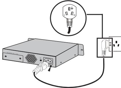
Figure 3-4 Connecting to Power Supply
