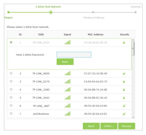
4) Either copy the host's SSID or customize it for 2.4GHz extended network, then click **Next**.
