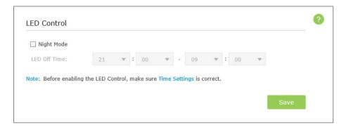
• **Night Mode:** If the Night Mode box is checked, all the LEDs are off in the setting time.
